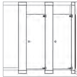
Floor to Ceiling Anchored
